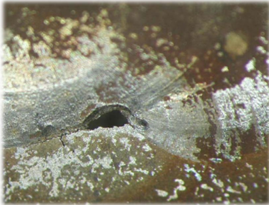
Fig.2. Inner surface of the section with the leak at the location of the melt line on the 2 mm side. The leak had a size of approx. 1 mm. Magnification: 25x.
