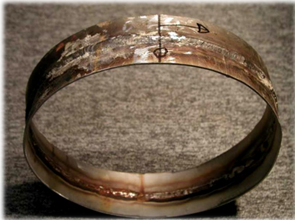
Fig. 1. Overview of the section with circular weld received for examination.
