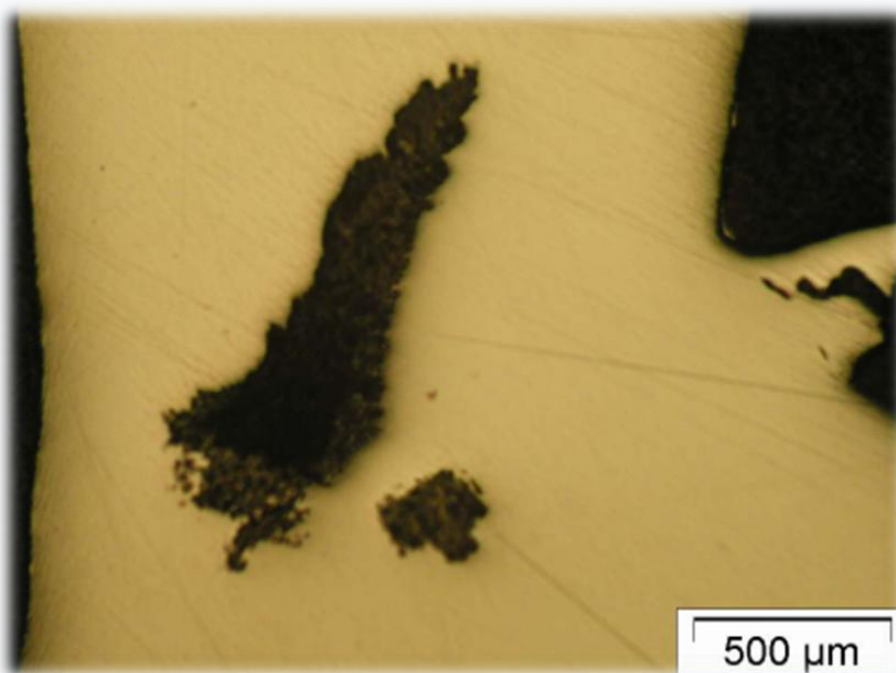
Fig.5. Cross-section next to the leak. The leak was undercut and filled with corrosion product.
