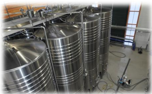
Stainless steel AISI 304 winetanks
