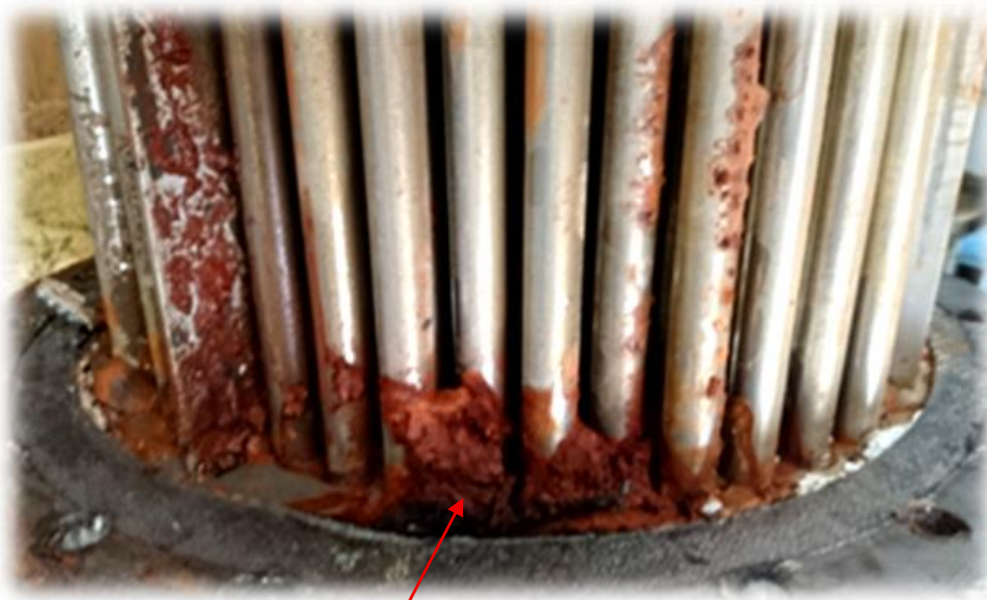
Clear form of microbiologic corrosion at the end of the tubes
