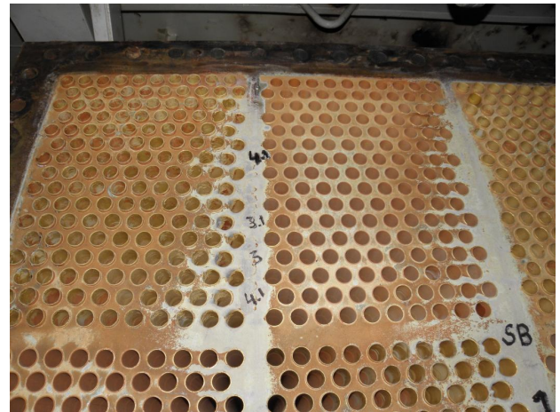
Maximum 4.1 mm tube sheet SB 1
