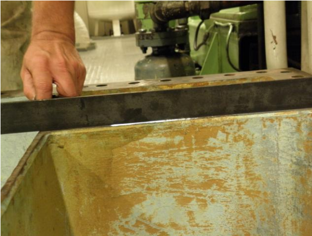
Space between ruler and marine box FDW \Delta 2mm
