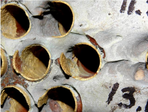
Tubes sheet thickness reduce till 13 mm
